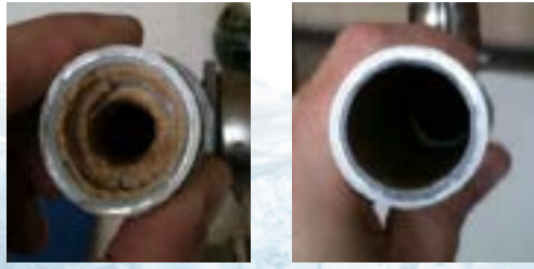
Conductor condition after three months of operation without and with AquaKat.
